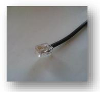
Please ensure that the coiled lead is plugged into the Nurse Call socket on the right hand side of the monitor and then either plugged into the Jack (if it's a stereo/mono connection), or plugged directly into the call system.
